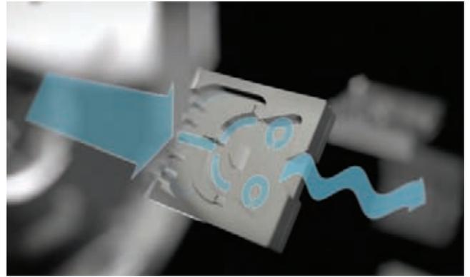
Each channel is designed to create a vortex that oscillates water and sculpts it as it exits into a wave pattern that provides a dense, concentrated spray—to give the feeling of an indulgent shower, without wasting water.
